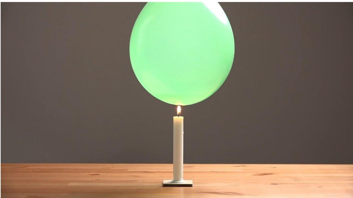
Figure 4: Heat resilient balloon due to heat capacity of water
